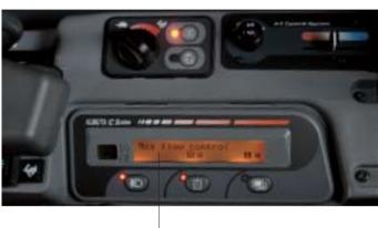
Kubota's KX080-3 is the first and the only mini/midi excavator to offer this unique and revolutionary feature. Combined with the Kubota Intelligent Control System, this function allows you to control the oil flow according to your needs or the attachment in use.
